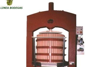
PRENSAS HIDRAULICAS CON MOTOR PHM
